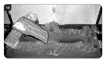
7.14 Place Log C on the right hand side of the burner. There is a hole on the underside of Log C which fits over the raised stud on the right of the burner. The back of the log should rest flush against the back panel, see Diagram 17.
