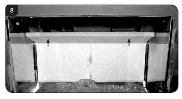
Once the baffles have been placed carefully to one side the liners can then been taken out in the following order.
